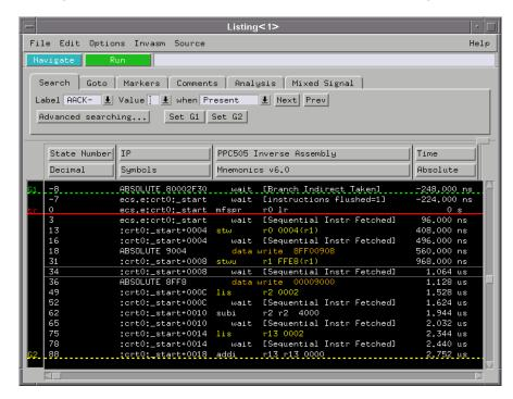
The inverse assembler is already loaded when state configuration files are loaded, but it can also be loaded into a Listing display using the Invasm menu.
