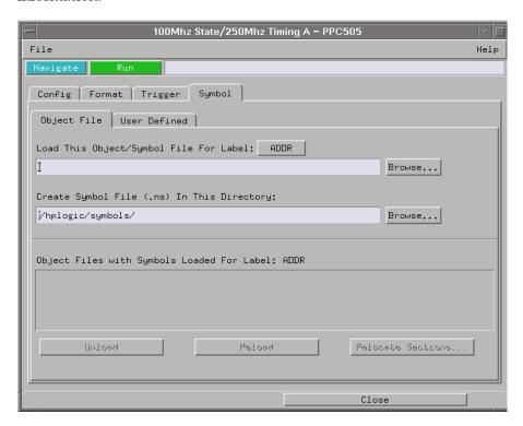
When you load object file symbols into a logic analyzer, a database of symbol/line number to address assignments is generated from the object file.
