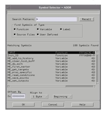
Entering the appropriate address offset will cause the logic analyzer to reference the correct symbol information for the relocatable or offset code.
