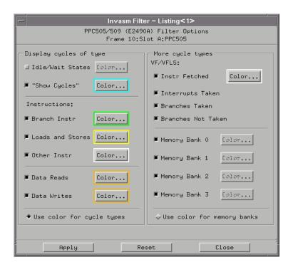
The inverse assembler filtering options allow you to display or hide certain types of microprocessor bus cycles or memory bank accesses.
